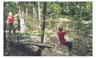
A bridge made from a single rope to walk on and another rope overhead to hold onto is a type of primitive suspension bridge often referred to as a monkey or Tibetan bridge.
