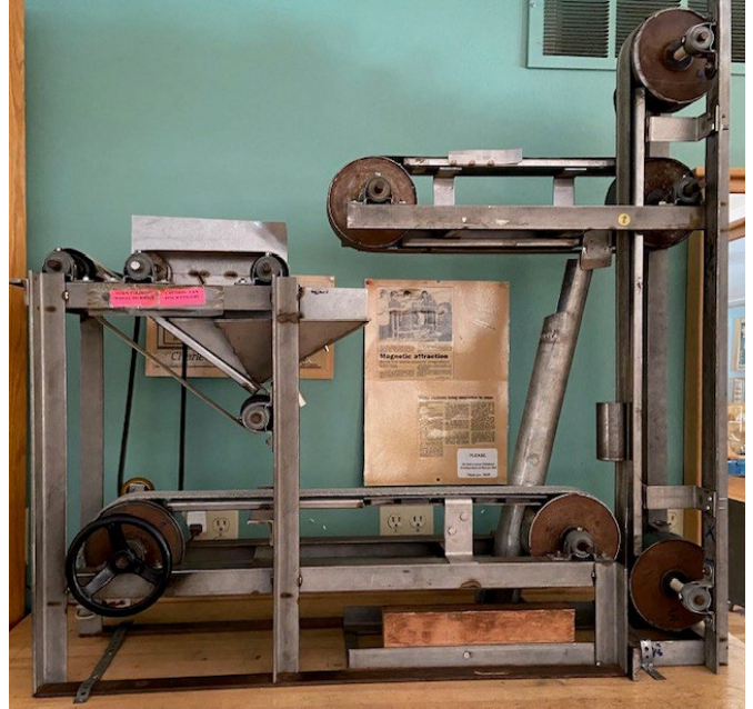
The final Magnet Machine consists of two sections, which can come apart. The vertical part rotates 90° and sits parallel to the horizontal piece for easy storage inside a cabinet. Be sure to give the Can Mover a try next time you visit Raven Hill. Be willing to help the can along the pathway, as needed.
