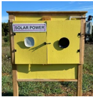
The black and white plates attached to the shutters on the Solar Station illustrate heat energy absorption. Feel them and you can understand why we wear light colors in the summer and darker colors in the winter. White and light colors reflect heat and keep us cool. Black and dark colors absorb heat energy and keep us warmer.
