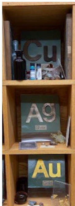
The gold symbol “Au” is actual “gold leaf”, which is a very thin sheet of gold—about 4 millionths of an inch thick—applied over base metal letters.
