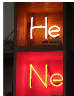
Helium and neon are two of the noble gases. They have 5000 volts of electricity applied to the gas in the tubes, which excites the electrons. The extra energy is given off as light.
