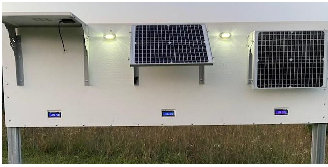
Slope kiosk displays 0-, 45- and 90-degree slopes and meters allow visitors to see the difference.
