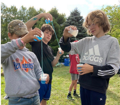
The polar nature of water, with its positive and negative “ends”, helps explain the surface tension of water and the ability to pour water down a string without it dripping.
