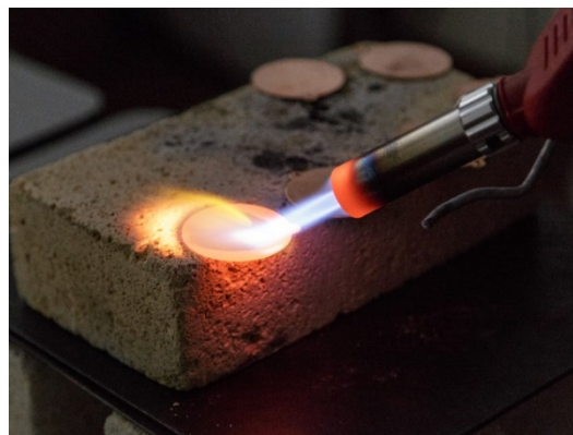
A propane torch replaces a camp fire in a more “modern” version of annealing or heating copper to make it more malleable and easier to shape.
