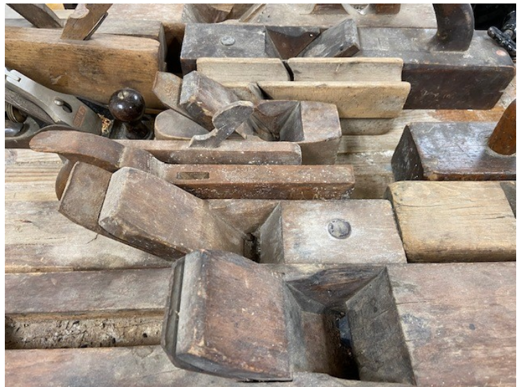
Traditional wooden hand planes smooth and shape wood. They come in many shapes and sizes. Once the metal and wood parts of these planes are cleaned and oiled, they will become part of the woodworking tool exhibit in the Wood Shop at Raven Hill.
