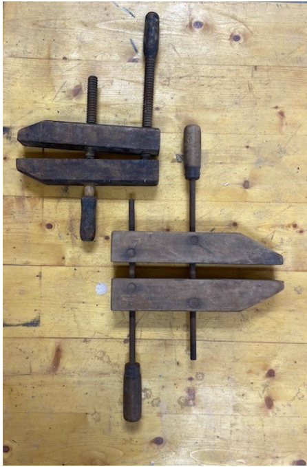
These wooden clamps look similar, but on closer inspection, one has wooden screws and the other has newer metal screws.
