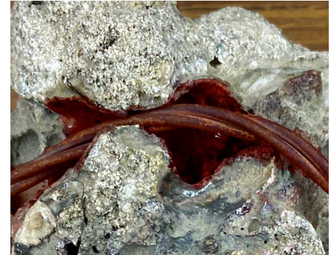
Close up picture of vitrified glass that formed, when this live copper wire fused the sand around it. Total size: 7"
