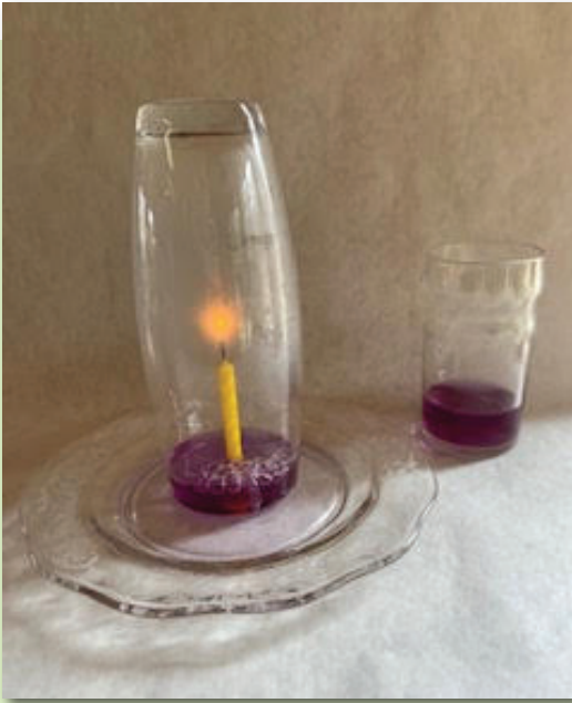
Air exerts pressure. More air outside pushes water into glass, where there is less pressure—flame uses up oxygen in air!
