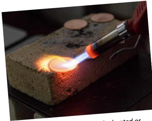
Copper pendants need to be heated or annealed before shaping.
