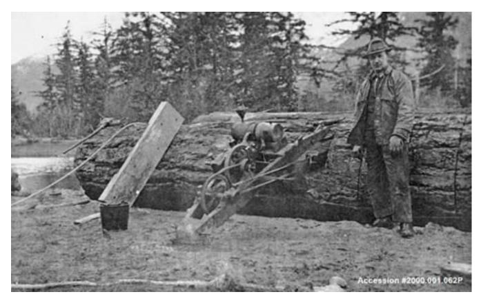
A dragsaw or drag saw is a large reciprocating saw using a long steel crosscut saw to cut logs to length. Prior to the popularization of the chainsaw during World War II, the dragsaw was a popular means of taking the hard work out of cutting wood. They would only work for a log on the ground. Dragsaws are known as the first mechanical saws to be used in the timber industry operation. These tools were most useful in the logging business, because they were efficient and very resilient.
