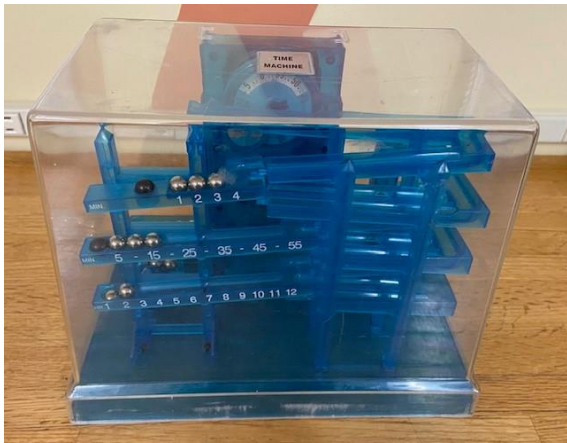
(Left) This Time Machine uses batteries, ramps, levers and steel bearing balls to keep time . Every minute a ball is released and rolls down a ramp. A fifth steel ball tilts the lever and the ball rolls into position to mark 5 minutes. After this happens 11 times (55 minutes), the next 5-minute ball marks 60 minutes, the ball tips the lever and a single ball rolls down to mark 1 hour or 60 minutes on the clock. Look closely and you can determine how many hours before the clock needs to be reset. —Raven Hill Collection
